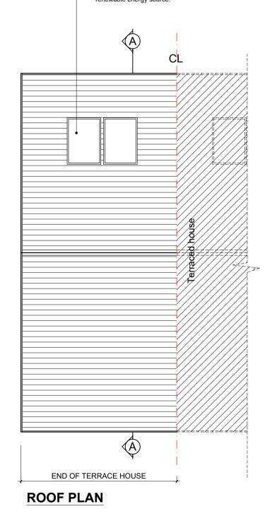
Indicitive Solar Panel Position, Final Solar Panel Position Depends on House Orientation The solar panels shown are a provisional option to satisfy renewable energy requirements of building regs part L. Solar panels may be omitted in favour of alternative renewable energy source.
